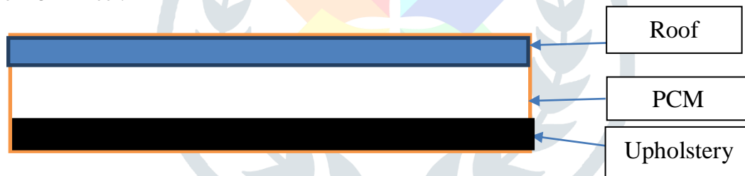
Figure 9: Configuration of PCM in roof
