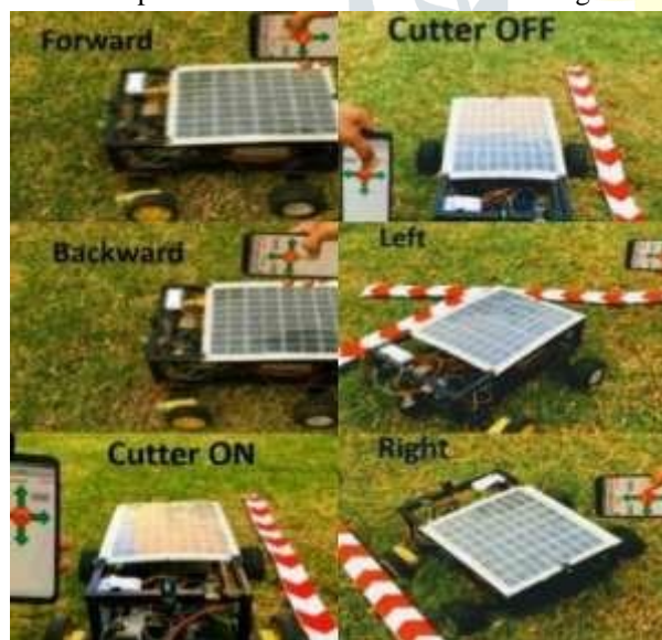
Figure 5: Different Movements of Grass Cutter The final demonstration of the proposed grass cutting robotic system with four different types of pattern like Circle, Spiral, Rectangle and Continue shapes designing on the grass is as shown in Figure 6.
