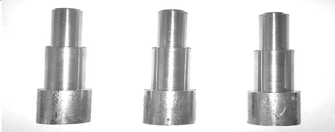
Fig 4.3 After operation of turning on AISI 316 Stainless Steel
