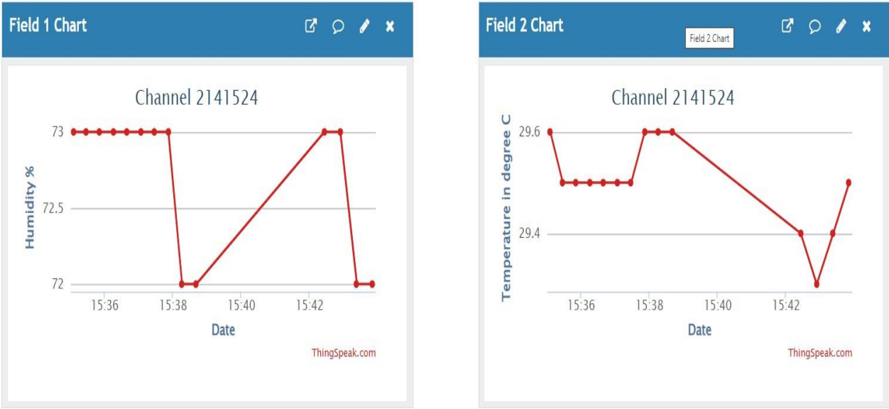
Figure 5: Result of ThingSpeak Field 1 and 2 for for humidity and temperature monitoring
