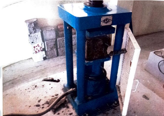
FIG 9: COMPRESSIVE STRENGTH TESTING ON PPCC
