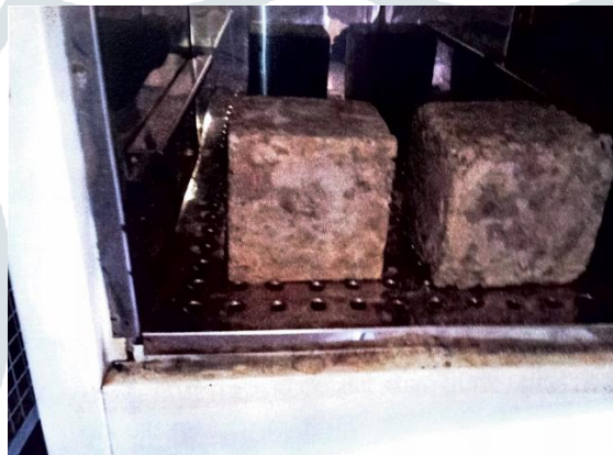
FIG 7: CURING OF GEO POLYMER CONCRETE 4.4 MIX DESIGN OF M-40 GRADE CEMENT
