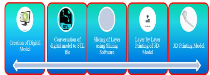
Figure 3. Steps in AM – Digital Model to 3D Model
