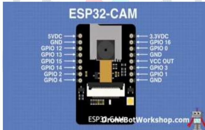
Figure 2.2: ESP32 camera pinout
