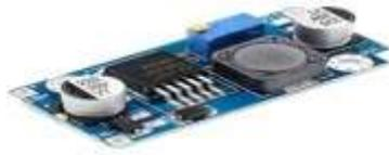
Figure 2.4: LM2596 DC to DC bulk converter
