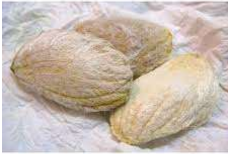
Fig 1 Mangifera indica shell used for coagulation
