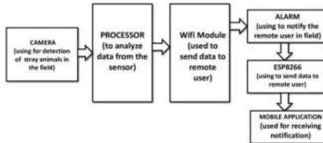
FIG.1 DETECTION AND MONITORING SYSTEM FOR STRAY ANIMALS
