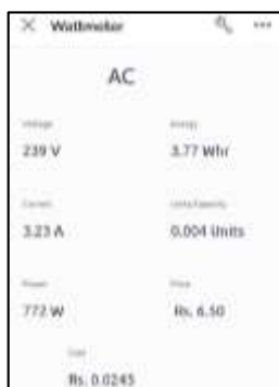
Fig. 6 Blynk mobile phone app screen showing readings of power consumption readings and total cost in rupees
