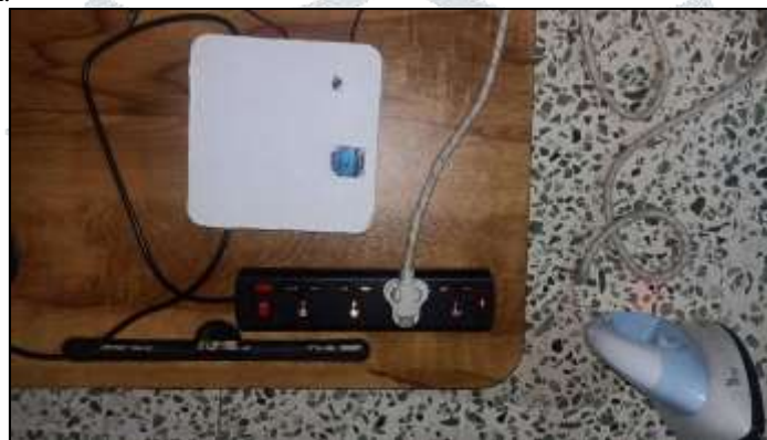
Fig. 5 Testing AC circuit of the energy meter with electric iron
