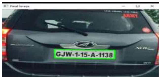
Fig.4-License Plate Localization being performed
