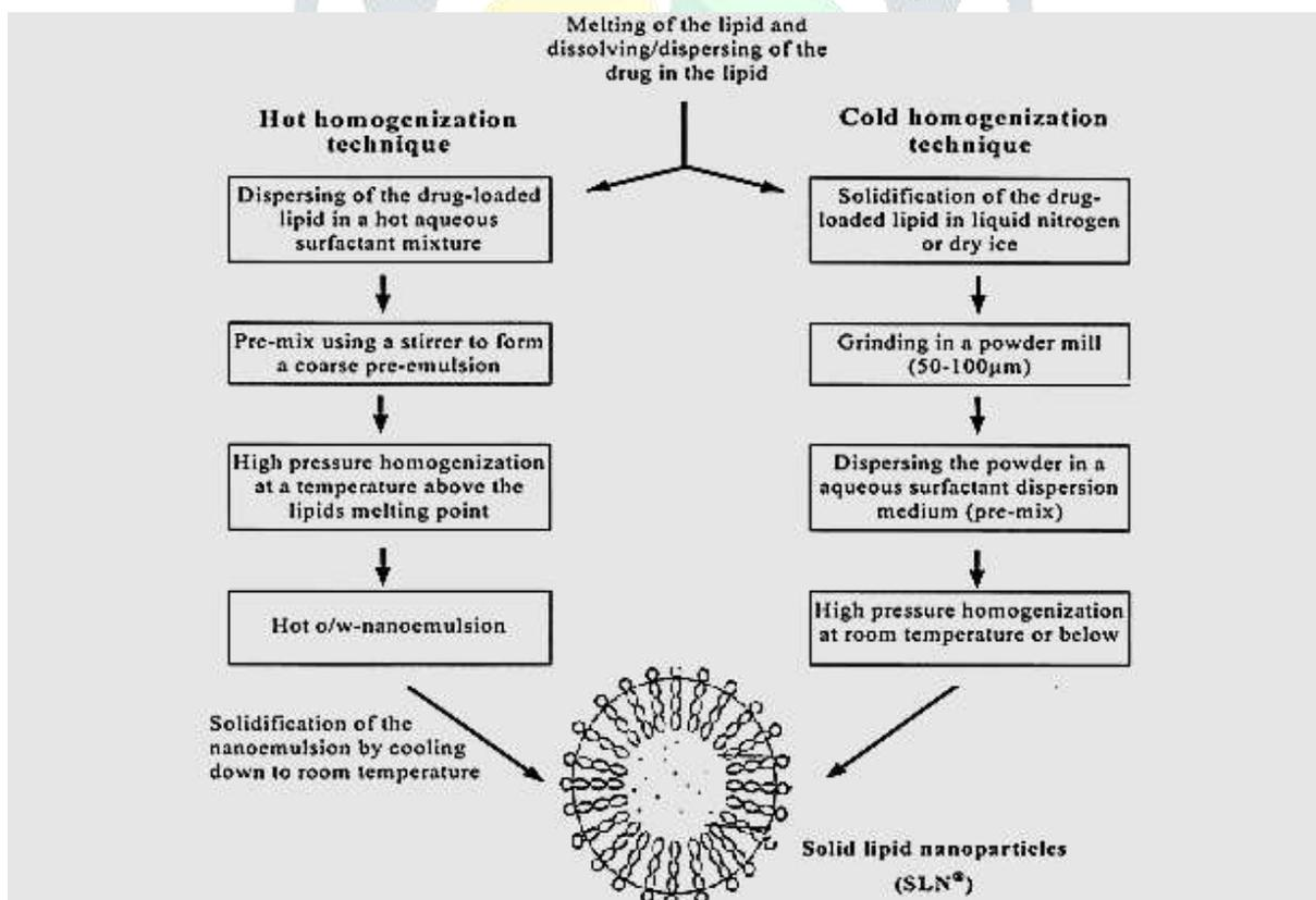
Fig. no. 6: Solid lipid nanoparticles preparation by hot homogenization process and cold homogenization process (R. Kabra et al., 2014).
