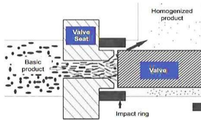
Fig. no. 5: Hot Pressure Homogenization (D. Ram et al., 2012).
