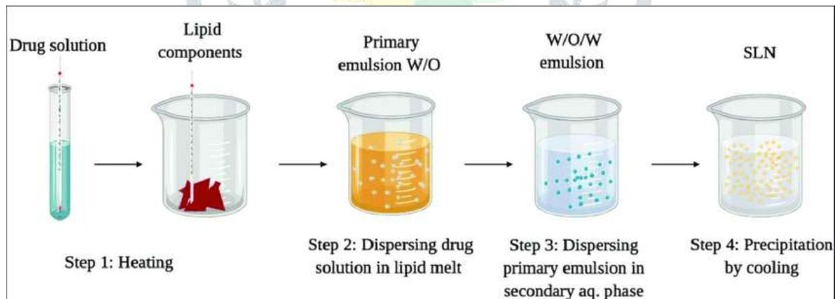
**Fig. no. 10:** Solid lipid nanoparticles preparation by double emulsion process (K. Sastri et al., 2020).
