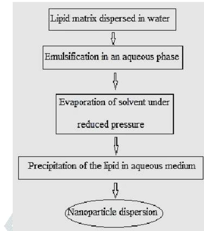
**Fig. no. 7:** Solid lipid nanoparticles preparation by Solvent evaporation process (P. Ekambaram et al., 2012).
