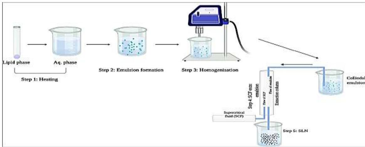
Fig. no. 8: Solid lipid nanoparticles preparation by Supercritical fluid method (K. Sastri et al., 2020).
