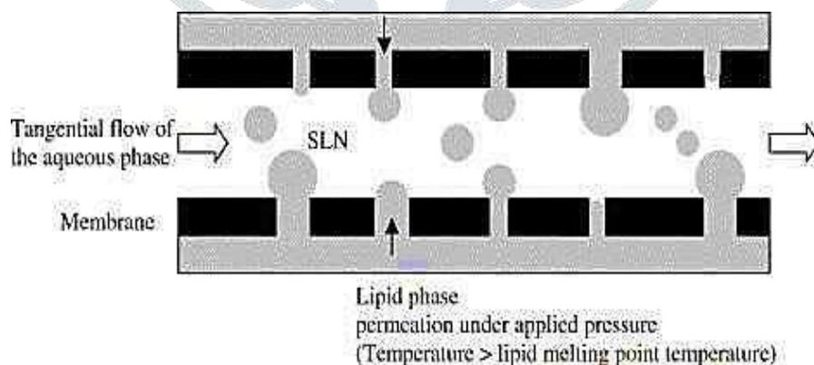
**Fig. no. 11:** Solid lipid nanoparticles preparation by Membrane contractor method (R. Parhi et al., 2010)
