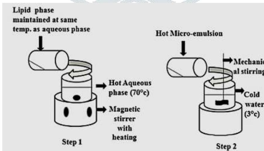
Fig. no. 9: Solid lipid nanoparticles preparation by Microemulsion based method (S. Bhatt et al., 2018)
