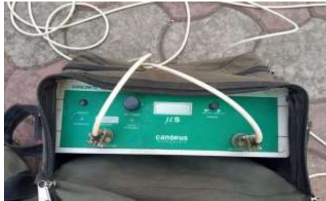
Figure 4 Ultra-sonic pulse velocity test
