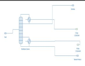
Fig 2. Process Flow Sheet for Simulated Rigorous Distillation Column for Benzene-Toluene System.
