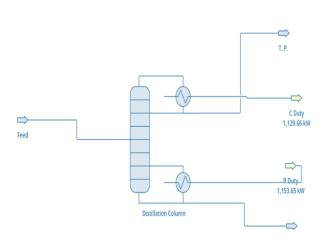
Fig1. Process Flow sheet for SC distillation Column for Benzene-Toluene System
