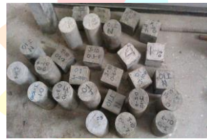
Fig 2. Fiber reinforced casted cubes
