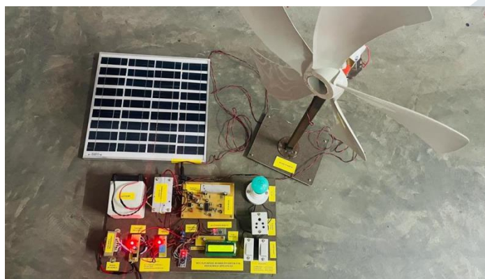
Fig5: Multi purpose hybrid inverter for household appliances with Load connected
