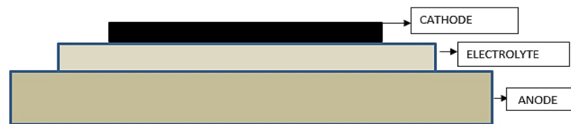
Figure 2: Cross Sectional view of the SOFC
