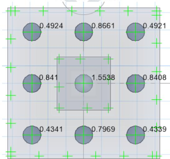
Fig 16: Pile foundation Punching Shear for 9 pile group.
