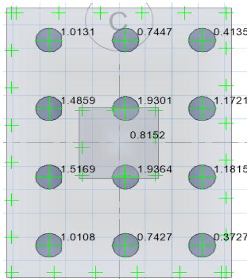
Fig 17: Pile foundation Punching Shear for 12 pile group
