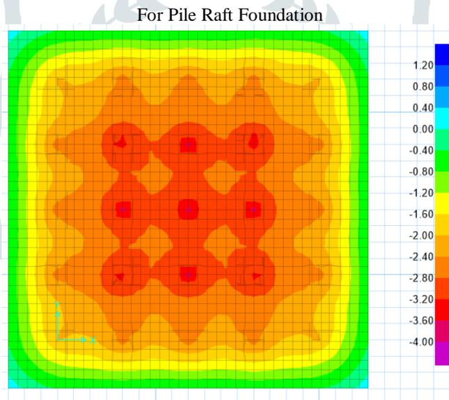
Fig 11: Pile Raft foundation Settlement
