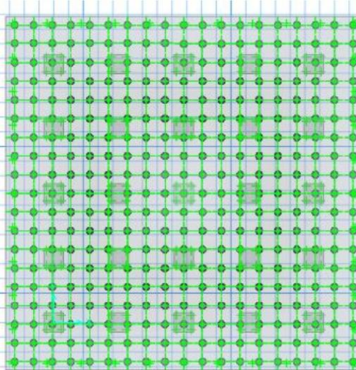
Fig 07: Finite Element Model of pile raft Foundation
