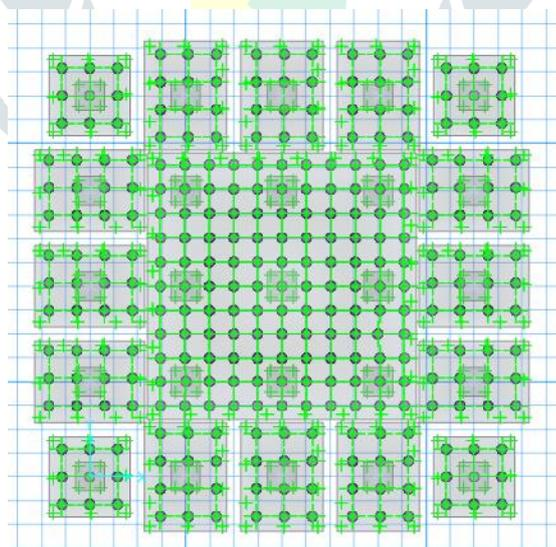
Fig 05: Finite Element Model of pile Foundation
