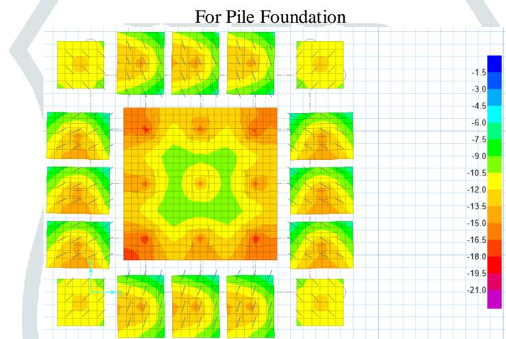
Fig 13: Pile foundation Soil Pressure Reaction
