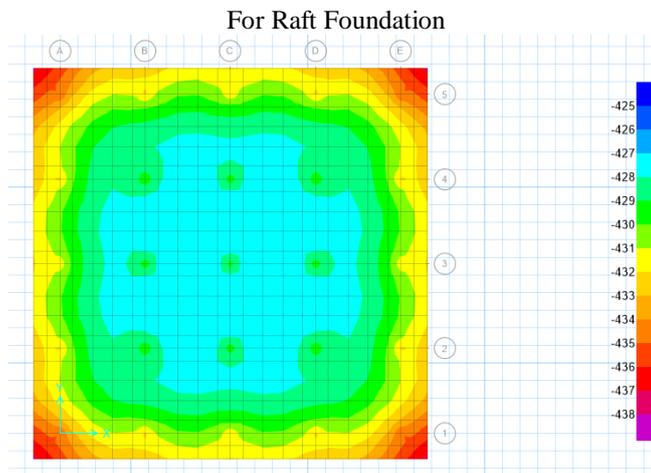
Fig 12: Raft foundation Soil Pressure Reaction
