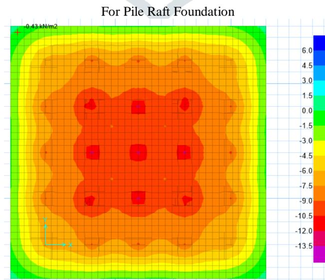
Fig 14: Pile Raft foundation Soil Pressure Reaction
