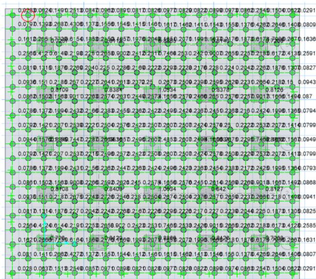
Fig 19: Pile raft foundation Punching Shear for 361 pile
