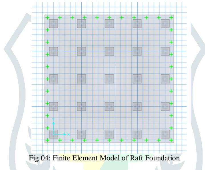
Fig 04: Finite Element Model of Raft Foundation
