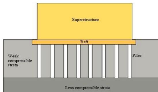
Fig 01: Piles with raft foundation.
