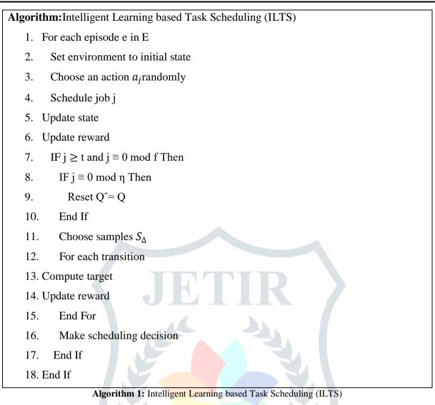
As presented in the proposed algorithm, it is observed that an agent has an iterative process as part of DRL to study action-space, state-space and reward function in making well informed decisions. The action taken by algorithm is given response in the form of reward. Then, the state transition takes pace. This process continues for each job to be scheduling until there is convergence which makes good decision that improves energy efficiency, success rate and also takes less execution time.
