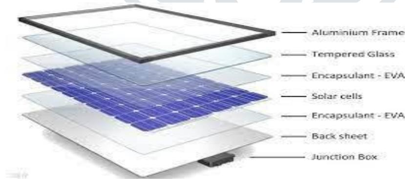
Figure 1 :- Layers of Solar panel
