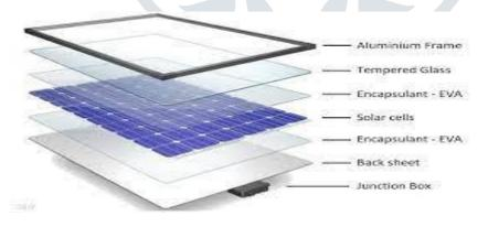
Figure 1 :- Layers of Solar panel
