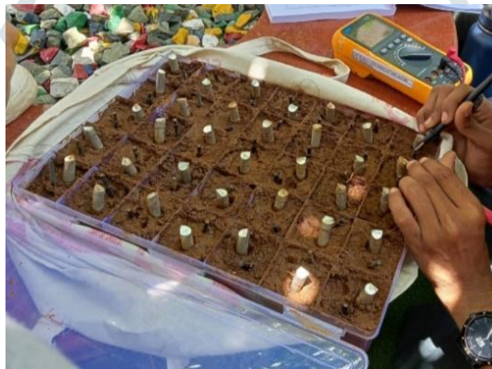
Fig.5 Testing of the prepared soil battery.
