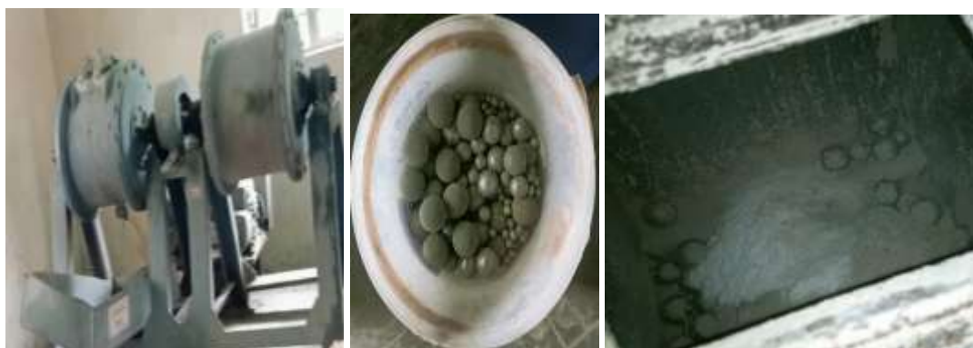
(a) Steel Ball mill with the balls
