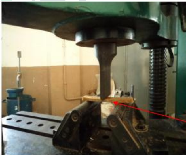
Fig -9: Experimental Set - Up for Flexural test
