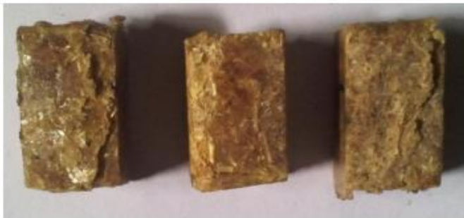
Fig -11: Tested compressive specimens
