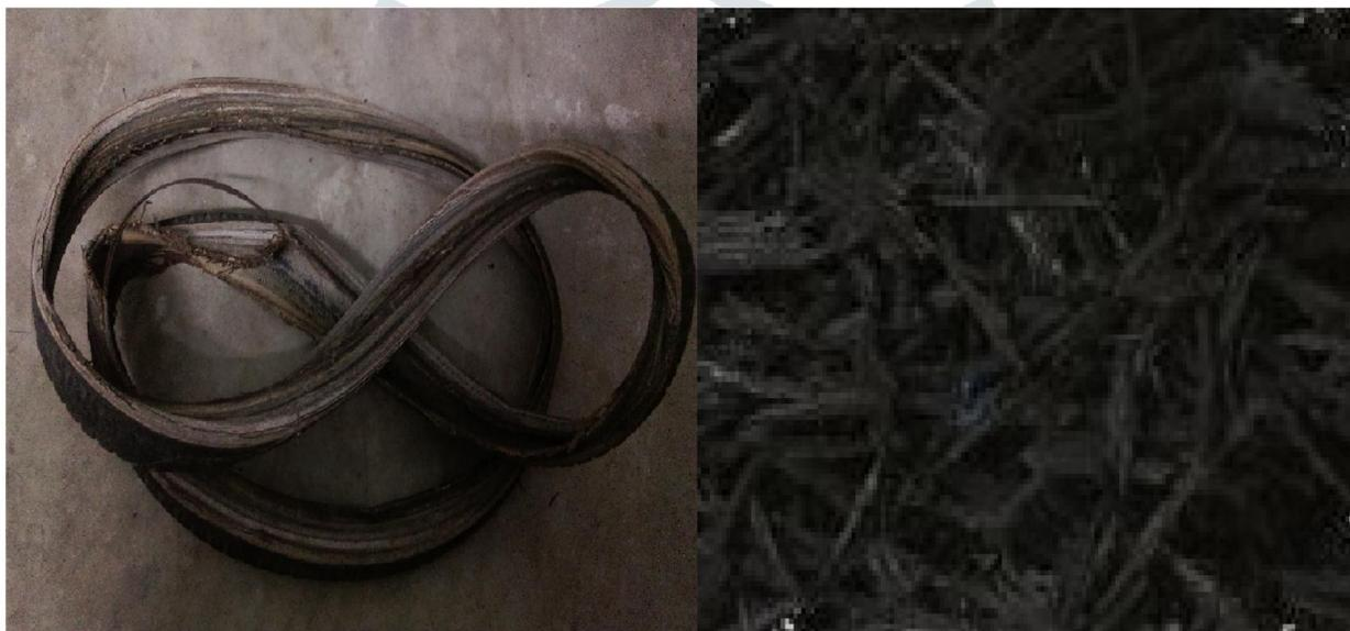
**Figure 3.2: Steel Wires Taken Out (Left) And Tire Cut In 30mm X 6mm (Right)**
