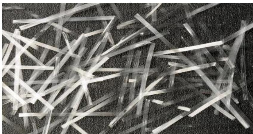
*Fig 1.3: Polyethylene Fiber (Source: Google Images)*
