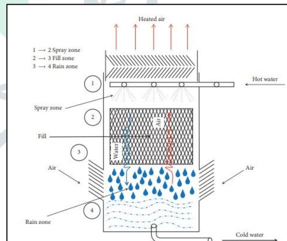
Figure 1: Schematic of a counter flow wet cooling tower [1]
