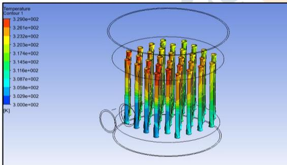
Figure 8: Temperature plot for water domain
