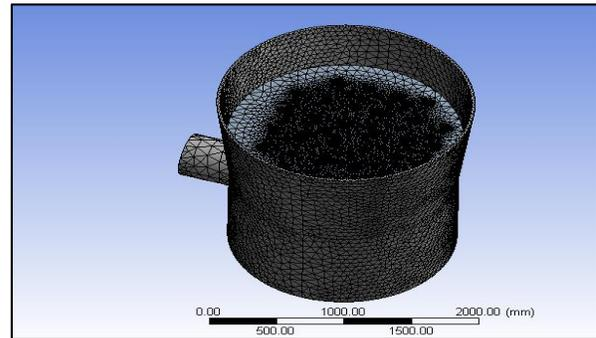
Figure 3: Discretized model of cooling tower
