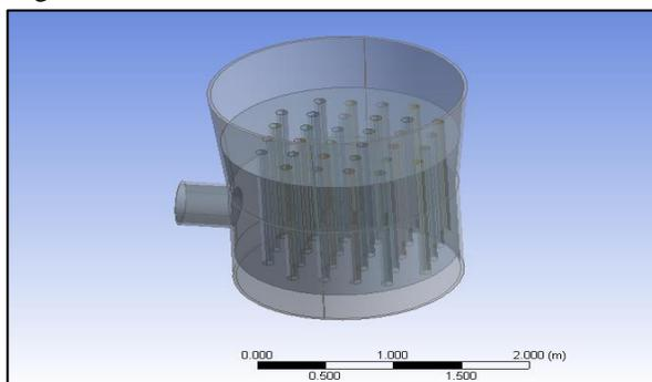
Figure 2: Imported cooling tower design in ANSYS design modeller
