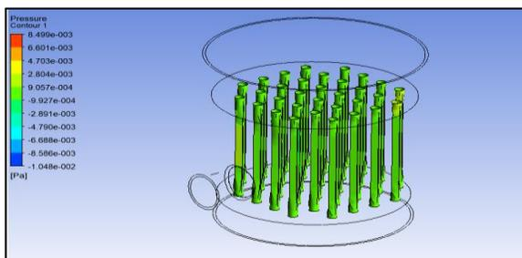
Figure 9: Pressure plot for water domain
