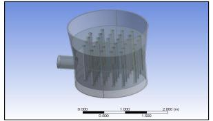
Figure 2: Imported cooling tower design in ANSYS design modeler
