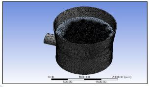
Figure 3: Discretized model of cooling tower
