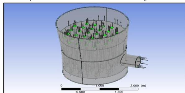
Figure 6: Water in boundary condition
