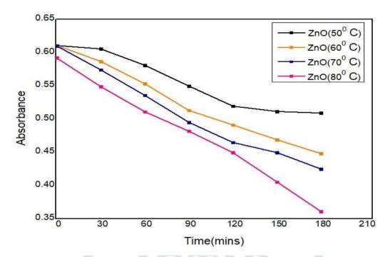
Fig.8. Degradation of ZnO nanoparticles at different temperature with regular time interval under UV irradiation
