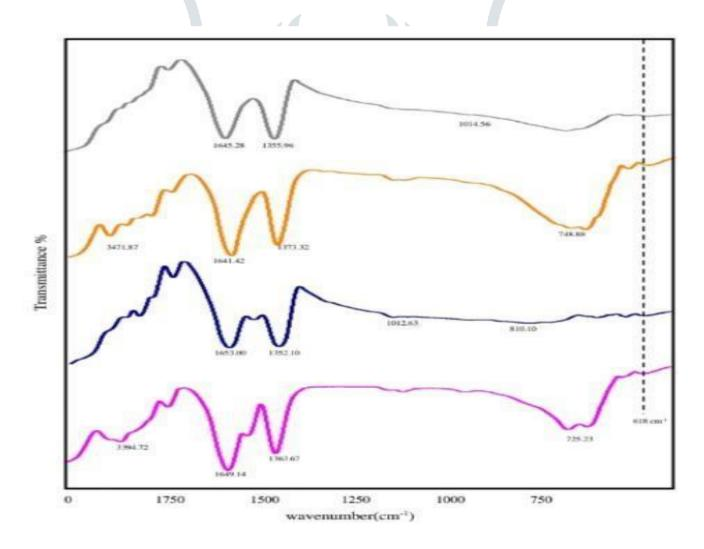
Fig. 4. FTIR analysis of ZnO nanoparticles at different temperature (50°C, 60°C, 70°C, 80°C)
