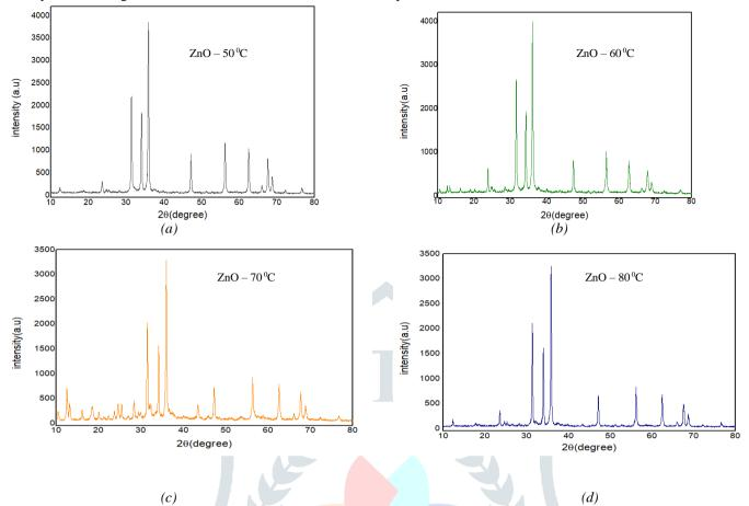
Fig. 2. XRD pattern of ZnO nanoparticles at different temperature ((a)50°C, (b) 60°C, (c)70°C, (d) 80°C)
