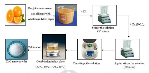
Fig.1. Schematic diagram of the green synthesis of ZnO nanoparticles
