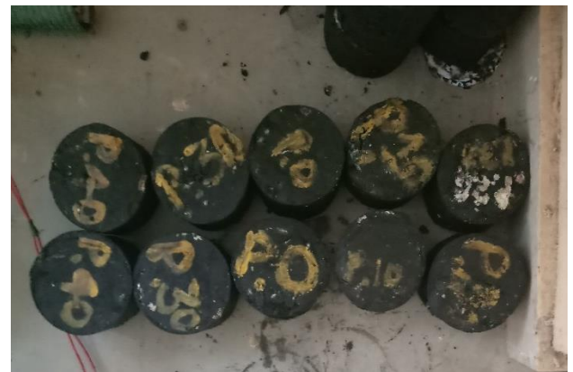
Fig 6 Prepared Marshall moulds
