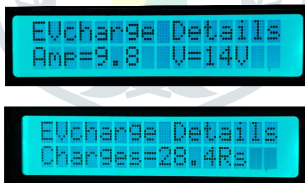
Fig. 11. Various charging parameters' visual output on display
