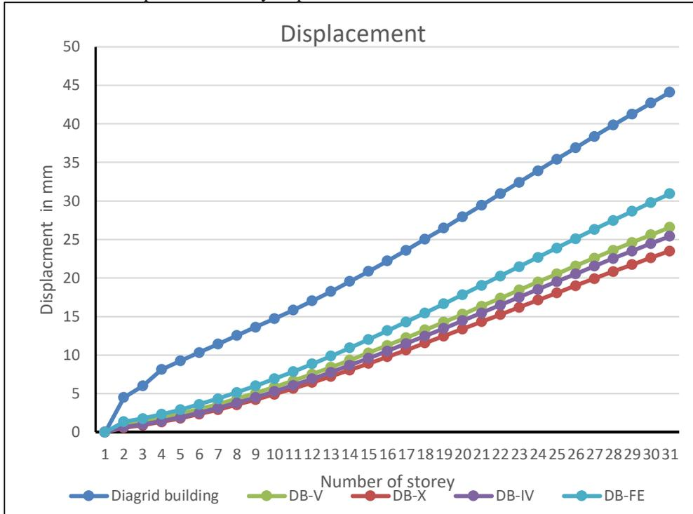
Fig 1.6 Comparison of storey displacement of all models.
