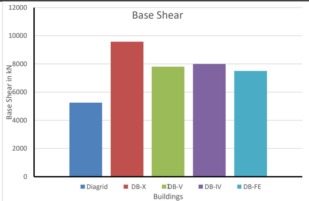
Fig 1.8 Comparison of base shear of all models.
