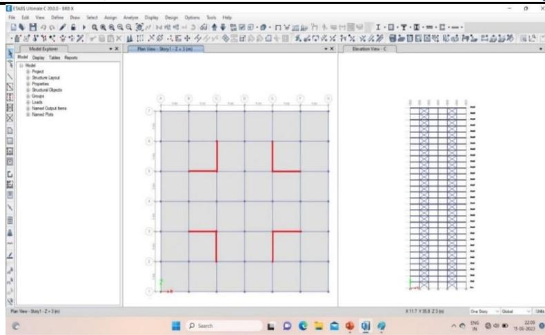
Fig 1.2 Diagrid building with X-arrangement of secondary bracing.
