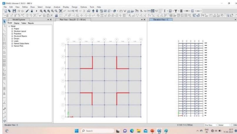
Fig 1.3 Diagrid building with V-arrangement of secondary bracing.
