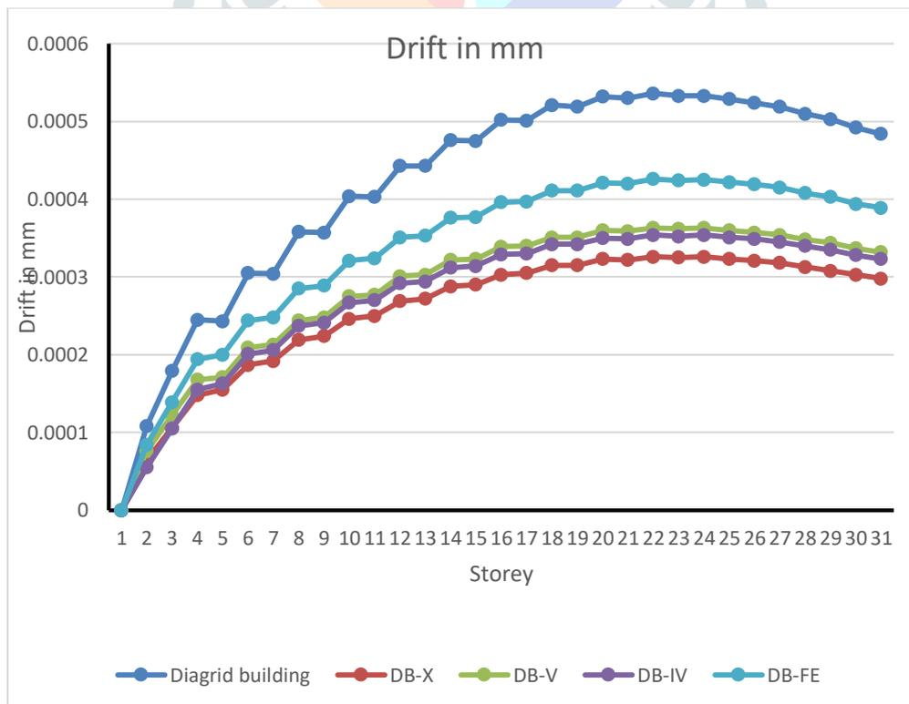
Fig 1.7 Comparison of storey drift of all models.
