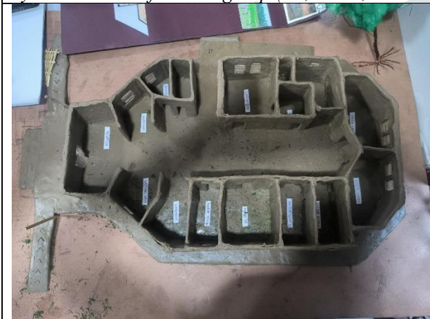
Figure 11 & 12 above: Finished models of rural health care facility in improvised wattle and daub walling with wooden truss supporting a green roofing, model showcasing all the layers of roofing with a monitor roof admitting light and air by the Students of control group (1A, USAP, GGSIPU, session 2022-23)
