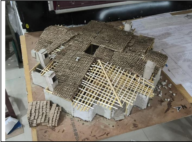
Figure 15& 16 above: Finished models of craft training facility in rammed earth walling with air catching shafts having bamboo truss supporting clay tiled roofing and rural granary and market in bamboo piers supporting a dynamic hyperboloid paraboloid bamboo roofing by the students of control group (1A, USAP, GGSIPU, session 2022-23)
