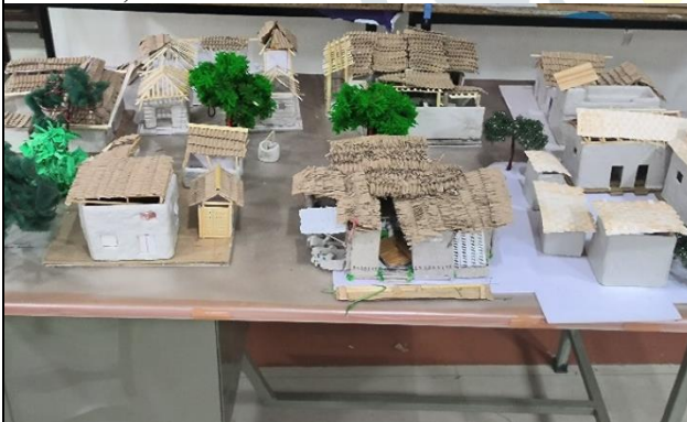
Figure 17 & 18 above: Finished models of craft training facility in bamboo piers supporting a butterfly truss and bamboo mat envelop roof covering by the students of control group (1A, USAP, GGSIPU, session 2022-23)
