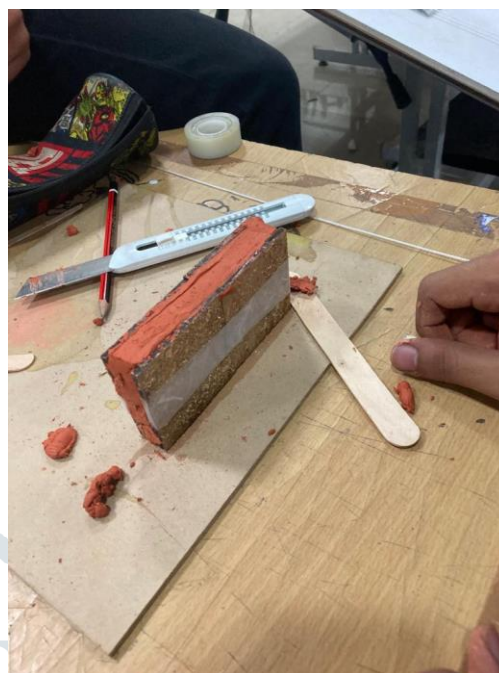
Figure 1 & 2 above: Initial process of walling techniques (Rammed earth ) modelled as per the processes true to construction of ramming and building in sections of 1.2m high at one time, by the Students of control group (1A, USAP, GGSIPU, session 2022-23)
