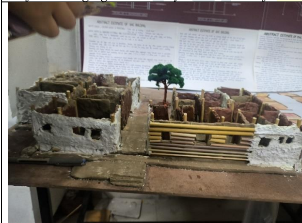
Figure 13 & 14 above: Finished models of rural health care facility in mud walling with bamboo split layers as support on both sides having a bamboo truss supporting a flattened split bamboo roofing envelop by the students of control group (1A, USAP, GGSIPU, session 2022-23)
