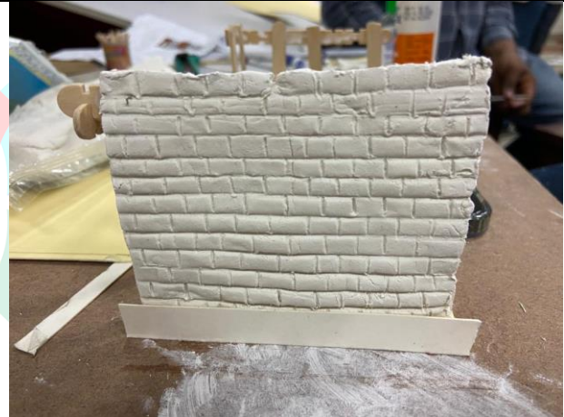
Figure 3 & 4 above: Initial process of walling techniques (Cob Walling Technique and Adobe walling technique) modelled as per the processes true to construction by the Students of control group (1A, USAP, GGSIPU, session 2022-23)
