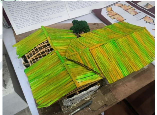
Figure 13 & 14 above: Finished models of rural health care facility in mud walling with bamboo split layers as support on both sides having a bamboo truss supporting a flattened split bamboo roofing envelop by the students of control group (1A, USAP, GGSIPU, session 2022-23)
