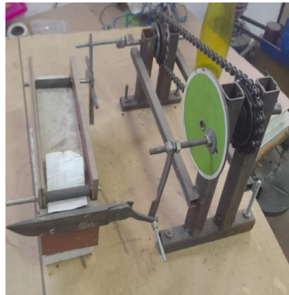
Figure no. 4.1 Diy Auto Paper Cutting Machine
