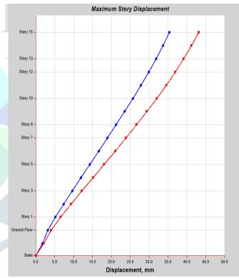
Fig 20. Maximum Story Displacement of Model I
