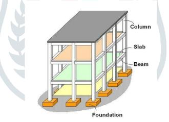
Fig.1 RC Conventional structure
