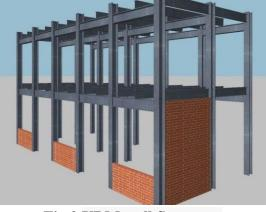
Fig.2 URM wall Structure
