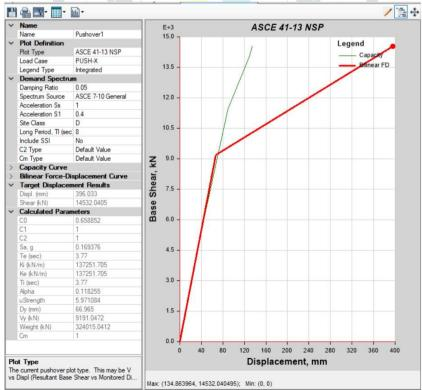
Fig 27. Target Displacement Point Results from ASCE 41-13 NSP
