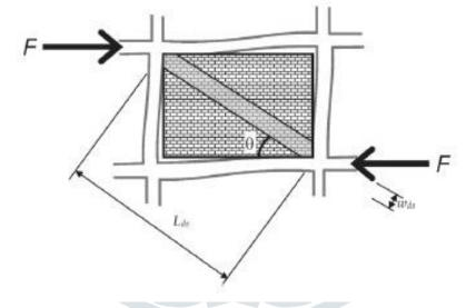
Fig 9. Equivalent Diagonal Strut of URM Infill Wall
