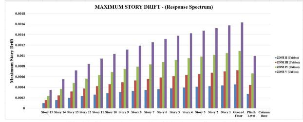
Fig 16. Comparison graph of Maximum Story Drift
