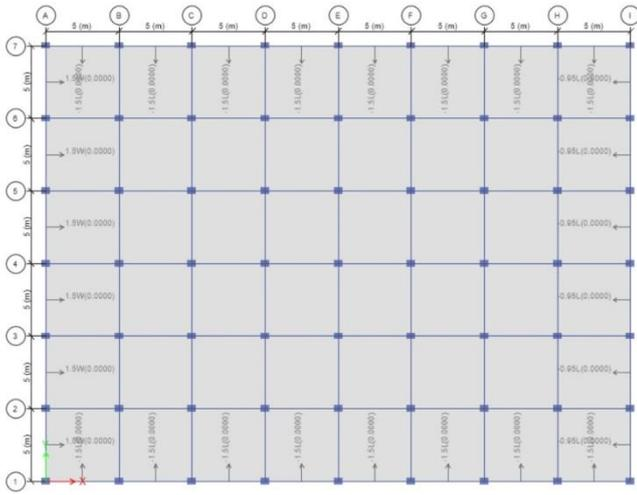
**Fig 7. Wind pressure co-efficients of structure**
