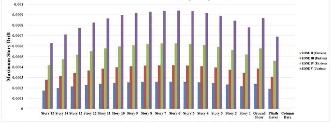
Fig 23. Comparison graph of Maximum Story Drift
