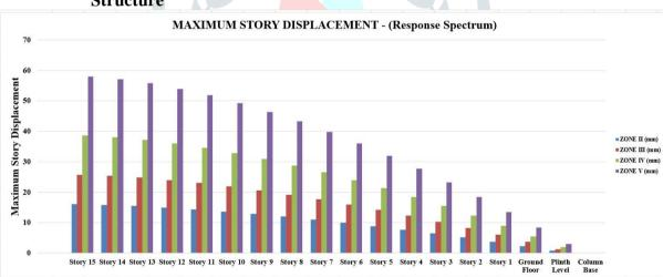
Fig 15. Comparison graph of Maximum Story Displacement 5.1.2. MAXIMUM STORY DRIFT- RC CONVENTIONAL STRUCTURE
