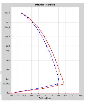
Fig 17. Maximum Story Drift of Model I
