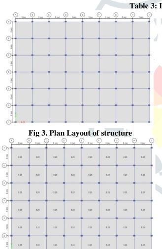
Fig 5. Dead Load on Slab
