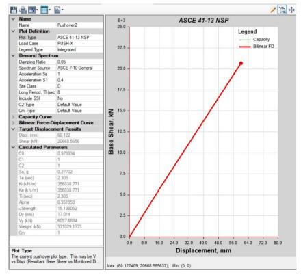
Fig 29. Target Displacement Point Results from ASCE 41-13 NSP
