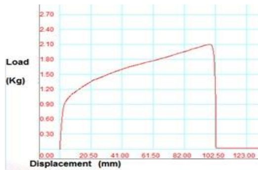
Fig 8: Pure PLA Load Vs Displacement Curve
