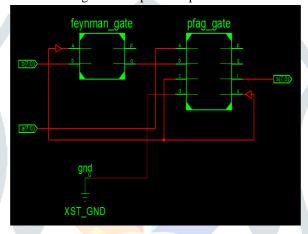
Figure 5: Proposed Reversible circuit using Feynman and Pfag Gate
