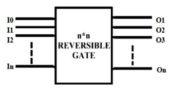
Figure 1: n\*n Reversible Logic Gate
