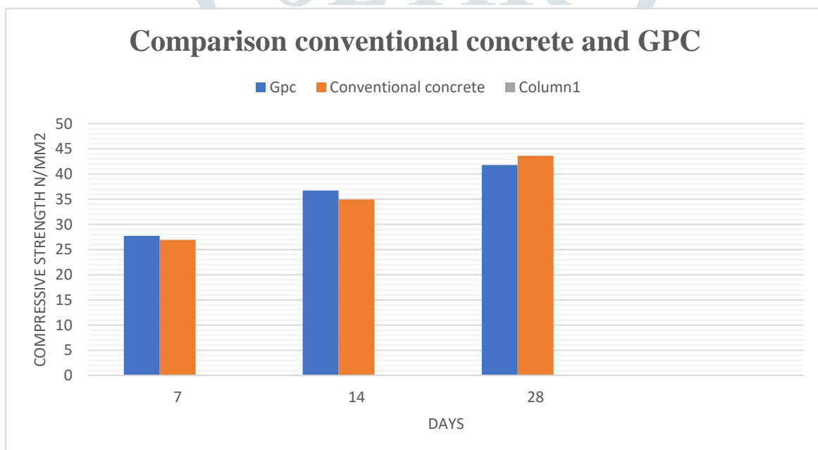
Graph 1-Comparison of compression strength of geopolymer concrete and conventional concrete.
