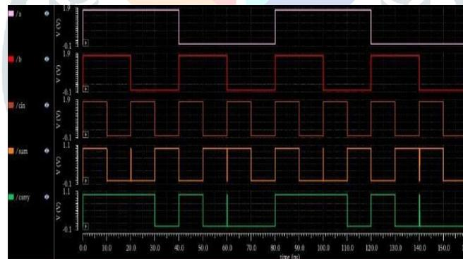
Fig.11. Full Adder Simulation result
