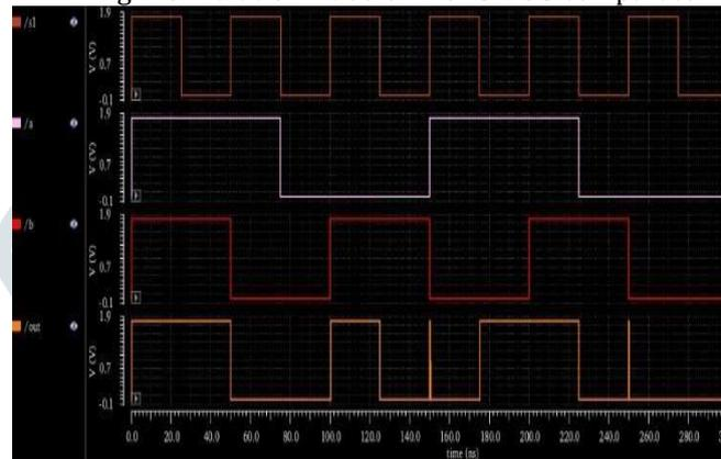
Fig.10. Multiplexer simulation result
