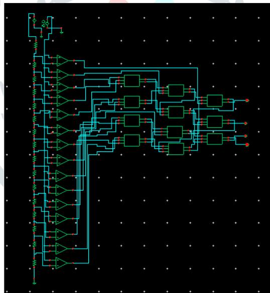
Fig.8. Schematic Diagram of Flash ADC
