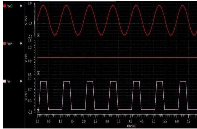
Fig.9. Simulation waveform of CMOS comparator
