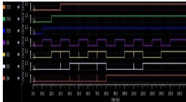
Fig.12. Simulation waveforms of Wallace Tree Encoder
