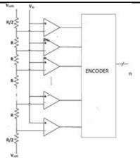
Fig.1. Flash ADC Architecture
