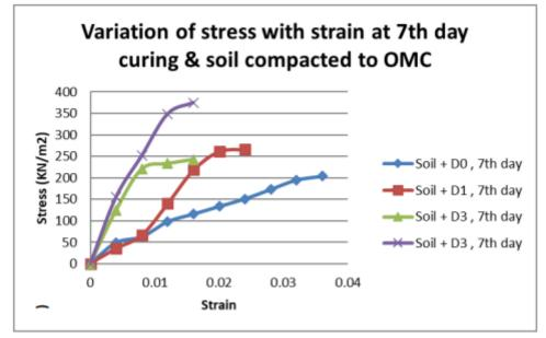
Fig 4. Variation of stress with strain at 7 day curing and soil compacted to OMC
