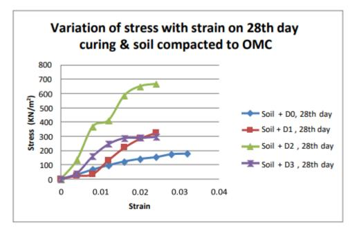
Fig 7. Variation of stress with strain at 28 day curing and soil compacted to OMC
