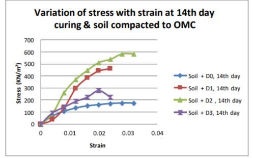
Fig 5. Variation of stress with strain at 14 day curing and soil compacted to OMC
