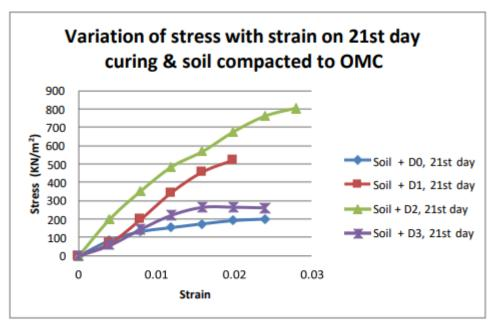
Fig 6. Variation of stress with strain at 21 day curing and soil compacted to OMC
