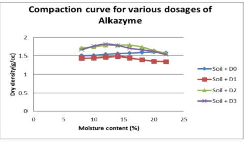
Fig. 2 Compaction curve for various dosage of Alkazyme
