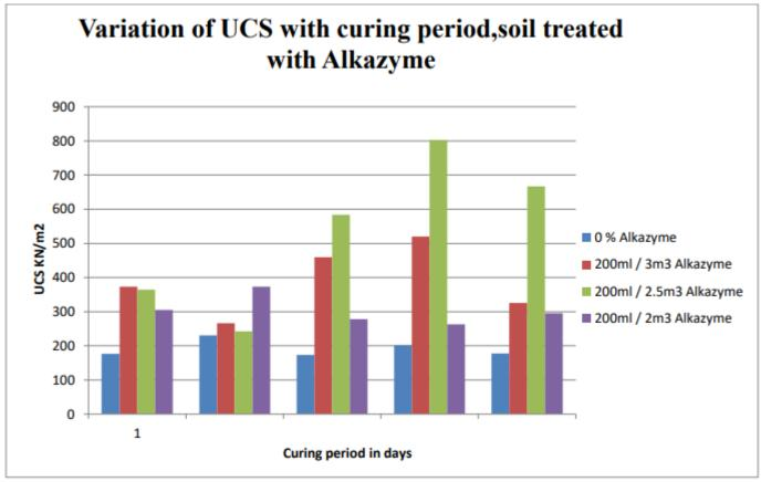
Fig 8. Variation of UCS with curing period, soil treated with Alkazyme
