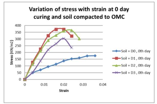
Fig 3. Variation of stress with strain at 0 day curing and soil compacted to OMC
