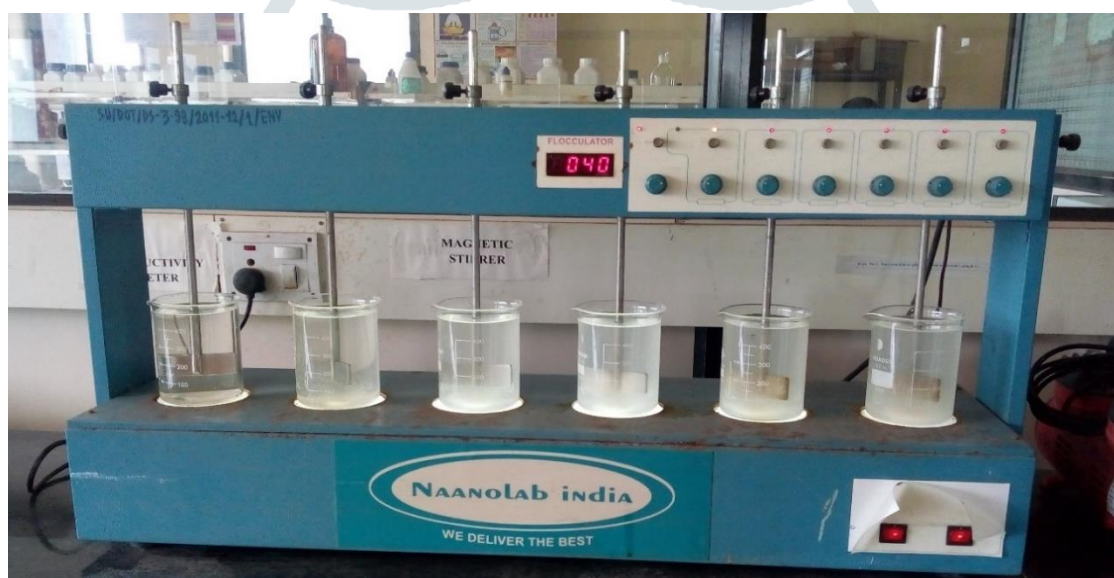
Fig. 4 Jar Test Using Natural Coagulant DOLICHOS LABLAB L (Indian Bean)
