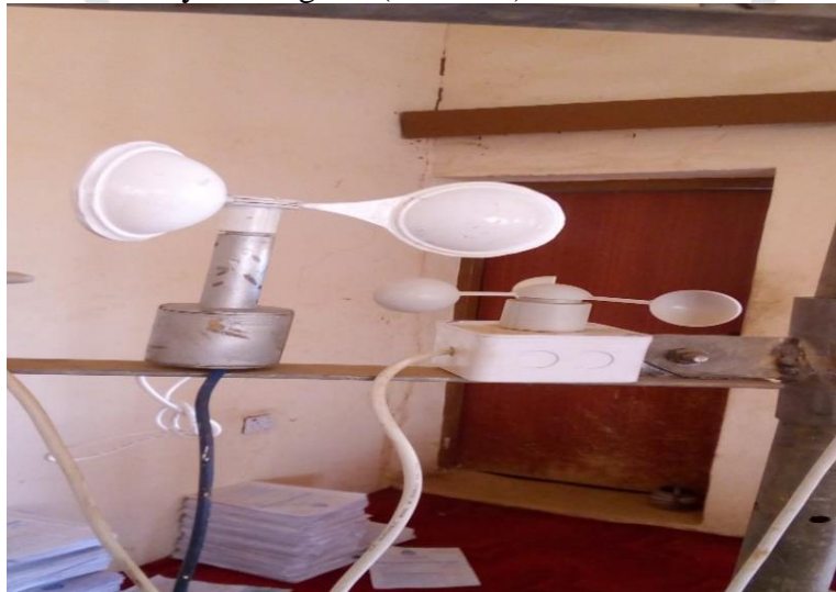
PLATE 2: SETUP TO CALIBRATE THE FABRICATED ANEMOMETER
