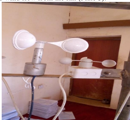
Plate 3: Set up of the accuracy test of fabricated anemometer
