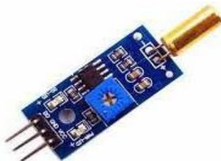
Fig1:- Tilt Sensor
