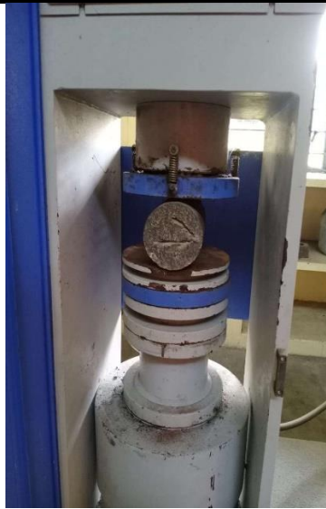
Fig 4: Split tensile strength test apparatus
