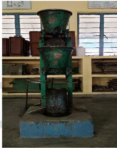
Fig 2: Compacting Factor test
