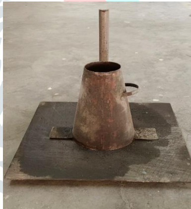
Fig 1: Slump cone Test
