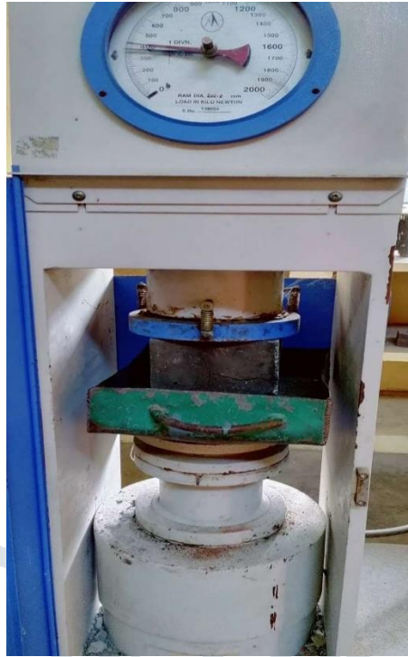
Fig 3: Compressive strength test apparatus
