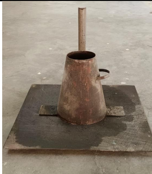
Fig 1: Slump cone Test
