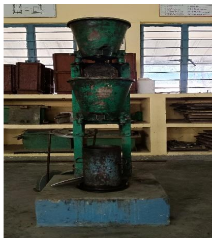
Fig 2: Compacting Factor test
