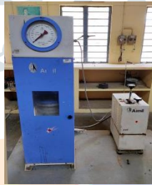
Fig 3 Experimental Set Up of Compressive Strength
