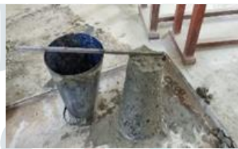
Fig 1 Slump cone Test
