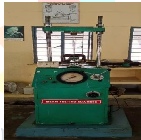
Fig 5 Beam testing machine
