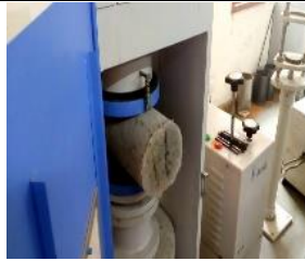
Fig 4 Experimental Set Up of Split Tensile Strength
