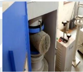
Fig 4 Experimental Set Up of Split Tensile Strength
