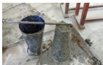
Fig 1 Slump cone Test
