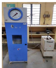
Fig 3 Experimental Set Up of Compressive Strength
