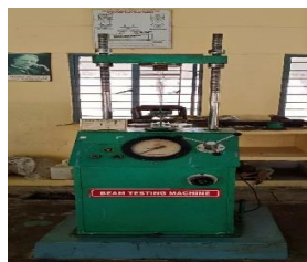
Fig 5 Beam testing machine
