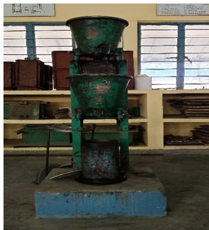
Fig 2: Compacting Factor test
