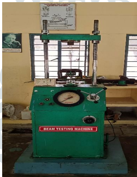
Fig 5: Beam testing machine
