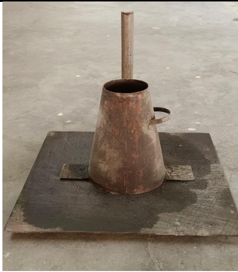
Fig 1: Slump cone Test
