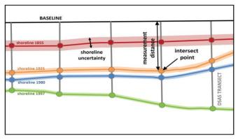
Figure 3 Components of DSAS tool
