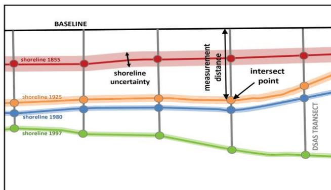
Figure 3 Components of DSAS tool
