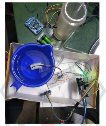
We will connect the LEDs and specify the voltage needed to alter the colours using analogWrite. A specific led will blink if the tank's empty level is more than 10 cm. In a similar vein, the second led will flash if the level is between 6 and 10 cm. Lastly, the last led will flash and the motor will also stop if the level is less than or equal to 3 cm. When the model is put to the test, the transition between the leds is clearly visible.
