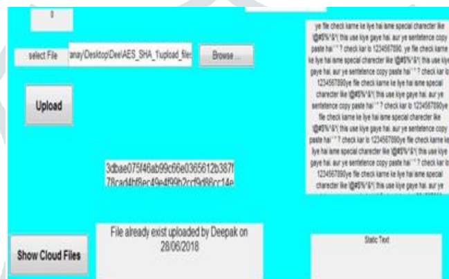
Fig. 4 (b) Shows Calculated Unique Hash Value And Shows File Already Exists Not Upload On Cloud
