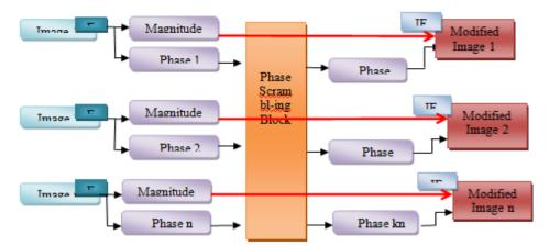
Fig. 2 Block Level Structure of Multiple Multimedia data (Image) encryption
