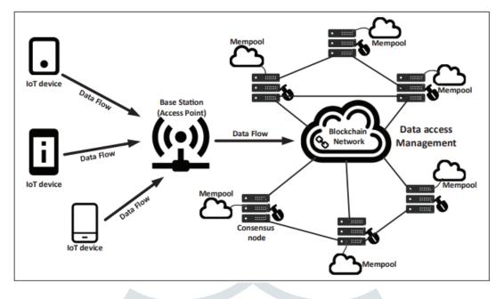
Figure 5: Schematics of blockchain-based transaction (data) transmission for IoT systems.
